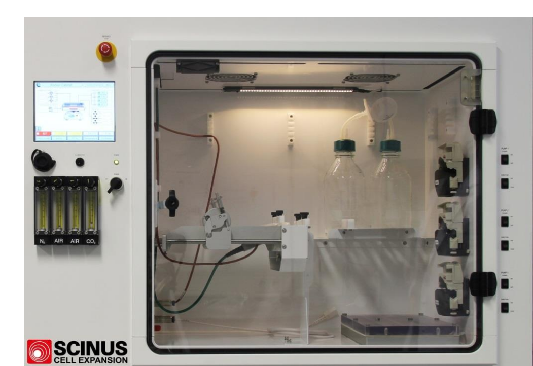
The Scinus Cell Expansion system, a closed bioreactor for cell therapy production
