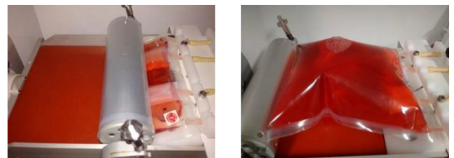
Figure 2 Expansion of the volume of the single-use bioreactor bag. Minimal volume (left) and maximum volume (right).
