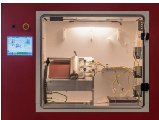
Figure 4 The Scinus Cell Expansion controller cabinet
