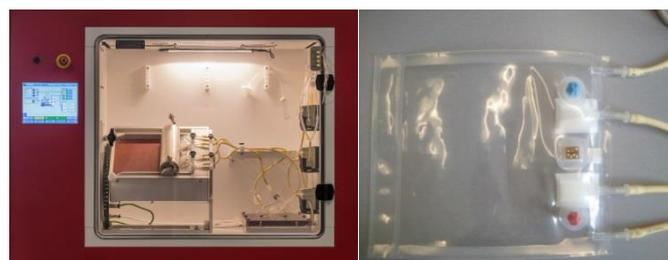
**Figure 1** The Scinus Cell Expansion system, consisting of a hardware cabinet enclosure (left) and a single-use bioreactor bag (right)
