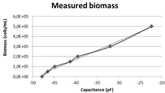
**Figure 3** Capacitance, as measured by the integrated biomass sensor, as predictor for cell concentration inside the bioreactor bag. Coefficient of determination,  $R^2=0.989$
